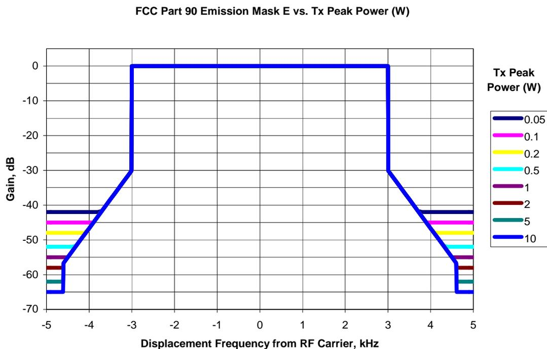
**Figure 1 FCC 90.210 Emission Mask E for Some Tx Powers from 50mW to 10W**
